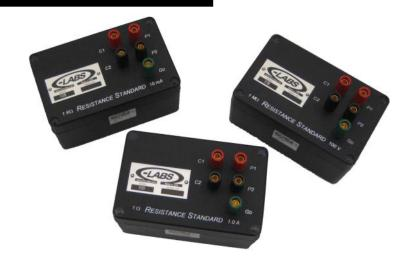
Ohm-Labs' 100-series resistance standards are designed for laboratory or on-site calibration. The low coefficients of temperature allow them to be used on a bench or in the field without loss of accuracy. They are immune from changes in barometric pressure and relative humidity, and are not affected by moderate vibration or shock. They display low reactance, allowing their use as both DC or AC standards.
