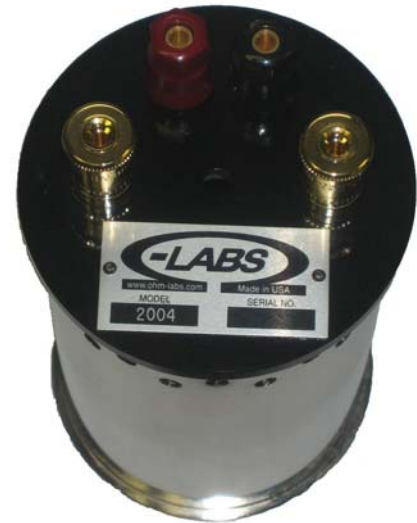
MODEL 2004 100 MICRO-OHM STANDARD
