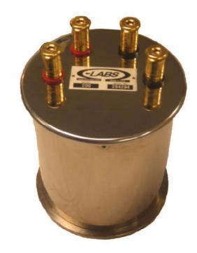
The Model 200 One Ohm Standard's rugged construction allows it to be used as a transport standard. Laboratories using Thomas type one ohm standards can keep these resistors in the laboratory and use the Model 200 as a transfer standard to a national laboratory or other reference lab.
